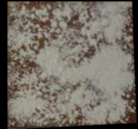
6: TiO2 sprinkled over finishing oil
